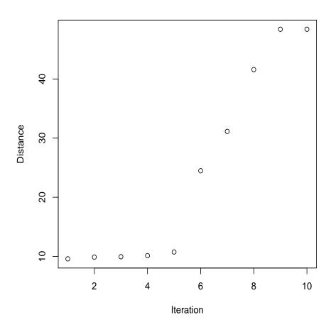
The change point Detection function can be used to find the change point in the chart of minimum distances and iterations to select the correct number of clusters. The MinIndex value indicates the index of the change point:
