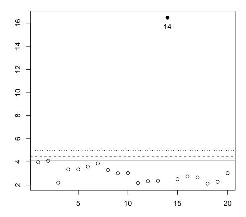
Figure 1: Results of MDQC based on all measures of the QC report. The MDs (y-axis) are computed using the robust S-estimator for each array (x-axis). The solid, dashed and dotted lines correspond to the square root of the 90th, 95th and 99th percentile of the Chi-Squared distribution, respectively. Outlying arrays are identified using solid points.
