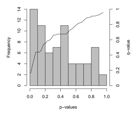
In this histogram the empirical p-values are drawn as usual in a histogram. In addition, the corresponding q-values corrected for multiple testing are plotted as a line into the histogram. The corresponding scale is shown to the left of the plot.
