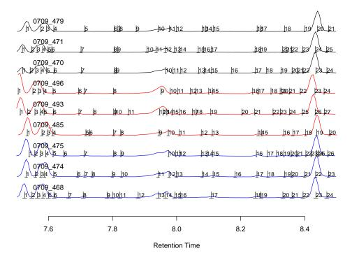
Note here the little *hashes* represent the detected peaks and are labeled with an integer index. One of the main challenges is to match these peak detections across several samples, given that the appear at slightly different times in different runs.
