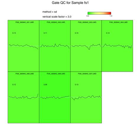
In this plot the fingerprints for each of the 7 tubes is shown in a grid. The color of the grid square for a tube indicates the standard deviation of the normalized and log-transformed fingerprint feature vector for that tube according to the color scale at the top of the figure. The standard deviation value is printed in the grid square.
