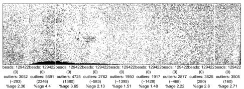
The artefact on the bottom edge of this strip can be seen clearly in both spatial plots. Such artefacts can be systematically detected and masked from further analysis using the BASH (beadarray subversion of Harshlight) tool. For details on how to use BASH, refer to the user guide which can be launched with the following command
